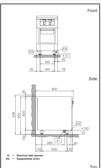
Electric Supply voltage: 400 V/3N ph/50/60 Hz Total Watts: 6 kW **Key Information:** 80 °C Working Temperature MIN: Working Temperature MAX: 350 °C External dimensions, Width: 500 mm External dimensions, Depth: 900 mm External dimensions, Height: 800 mm Net weight: 98 kg On Base;One-Side Operated Configuration: Sustainability
